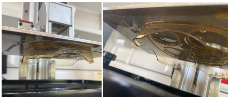
Figure 12. Photographs of the SLA printed nanocomposite prototype of an egg tray containing 0.5 wt % AgNO 3 .
