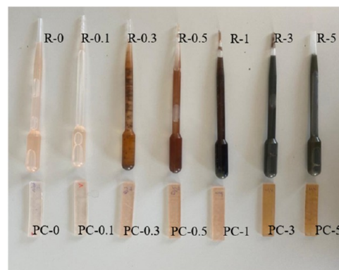
Figure 2. Photographs showing the neat and composite resins and printed specimens.
